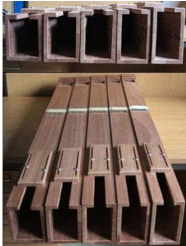
Fig. 2. Development of optimal scaling and a software for designing the depth and width of wooden organ pipes without changing the sound character
